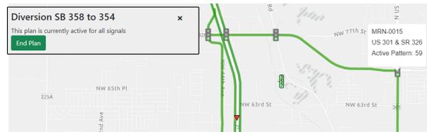
Figure 4: This southbound diversion modifies the active timing of 14 traffic signals in two jurisdictions.
